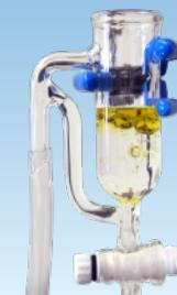
With conventional separation funnels, the liquid may overflow during the distillation. But by using the oil separator, the oil stays inside and the water is discharged through the bypass tube, which enables automatic separation.
