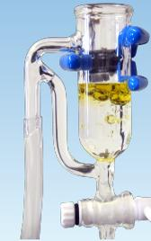
With conventional separation funnels, the liquid may overflow during the distillation. But by using the oil separator, the oil stays inside and the water is discharged through the bypass tube, which enables automatic separation.
