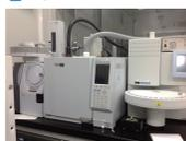
For the customers asking for more detailed distillation results and component distillation, we have begun the componential analysis service with GC-MS (gas chromatograph-mass spectrometer). It enables the column
